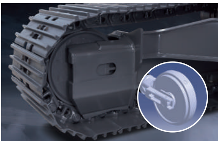
Integrated Track Spring and Idler The track spring and the idler have been joined directly to achieve high durability and improved maintenance convenience.
